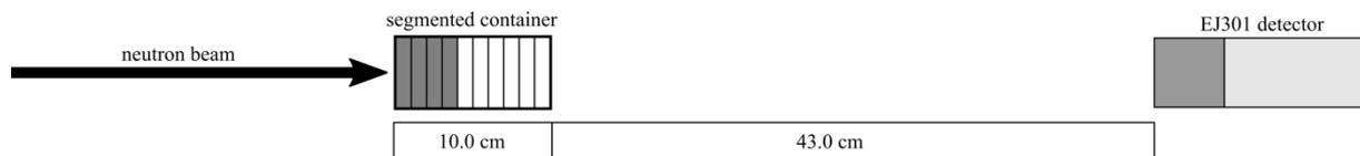
**Figure 1.** Fast neutron transmission experimental set-up. A pencil beam of  $^{241}\text{Am}$ - $^9\text{Be}$  neutrons is incident on the segmented container, where the shaded sections correspond to a measurement of 4.0 cm sample thickness. Transmitted neutrons are incident on a 2" x 2" EJ-301 organic liquid scintillator detector.
