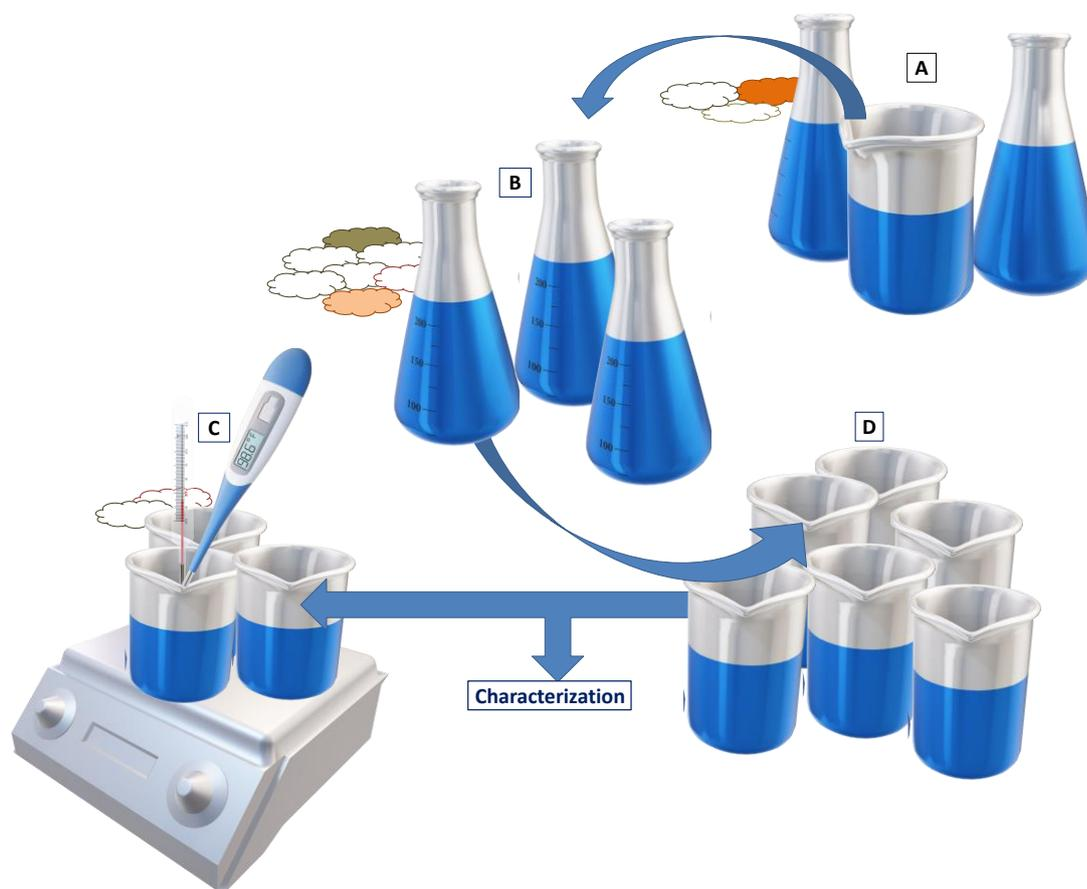
**Figure 1:** Synthetic experimental setup for synthesis of Au@SnO<sub>2</sub> nanocomposite structures. In the Figure, (A) Au seed synthesis, (B) Seed mediated growth of the nanostructures, (C) hydrothermal spontaneous encapsulation process of the Au nanostructures, and (D) the segmentation of the samples
