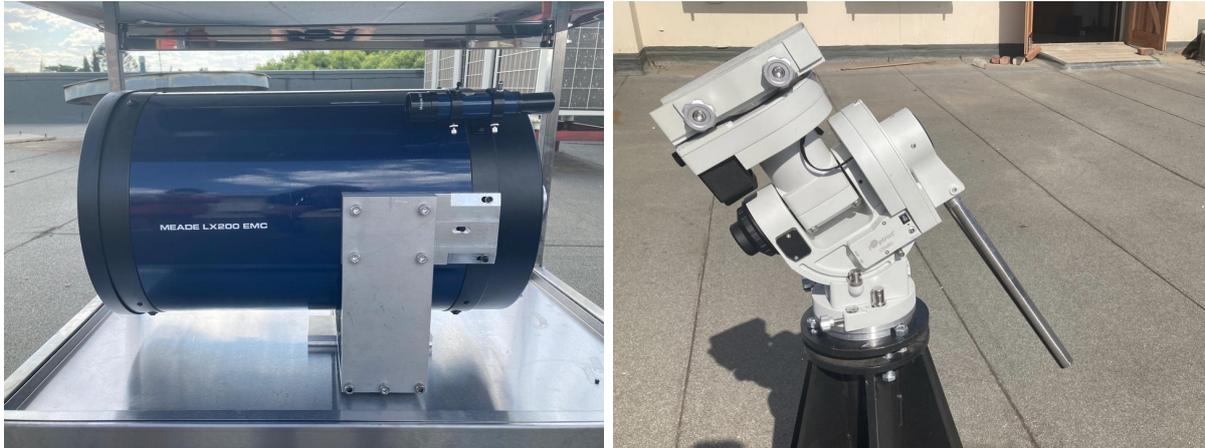
**Figure 1.** (a) The image shows the optical tube for the observatory. (b) The image of the iOptron CEM60 mount on the steel pier.
