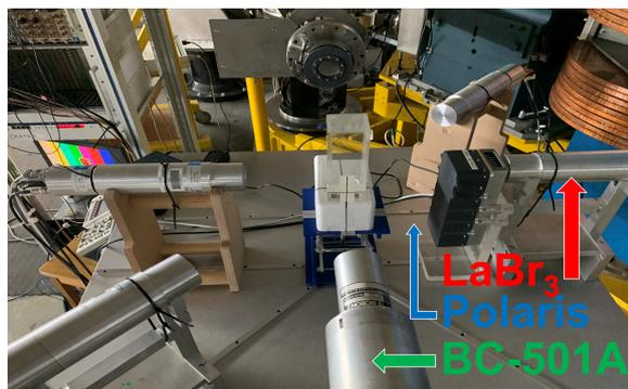
**Figure 5.** Detector configuration of 66 MeV proton incident on a water phantom
