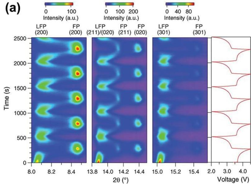
In situ XRD investigations performed on micrometer-sized  $\text{LiFePO}_4$  show the emergence of a metastable crystalline phase with an intermediate Li composition of  $\text{Li}_{0.6-0.75}\text{FePO}_4$  when cycled at high rates. Whereas, studies on nanometer-sized  $\text{LiFePO}_4$  particles are limited to low and moderate current rates, and only small deviations in stoichiometry from  $\text{LiFePO}_4$  and  $\text{FePO}_4$  were observed during cycling
