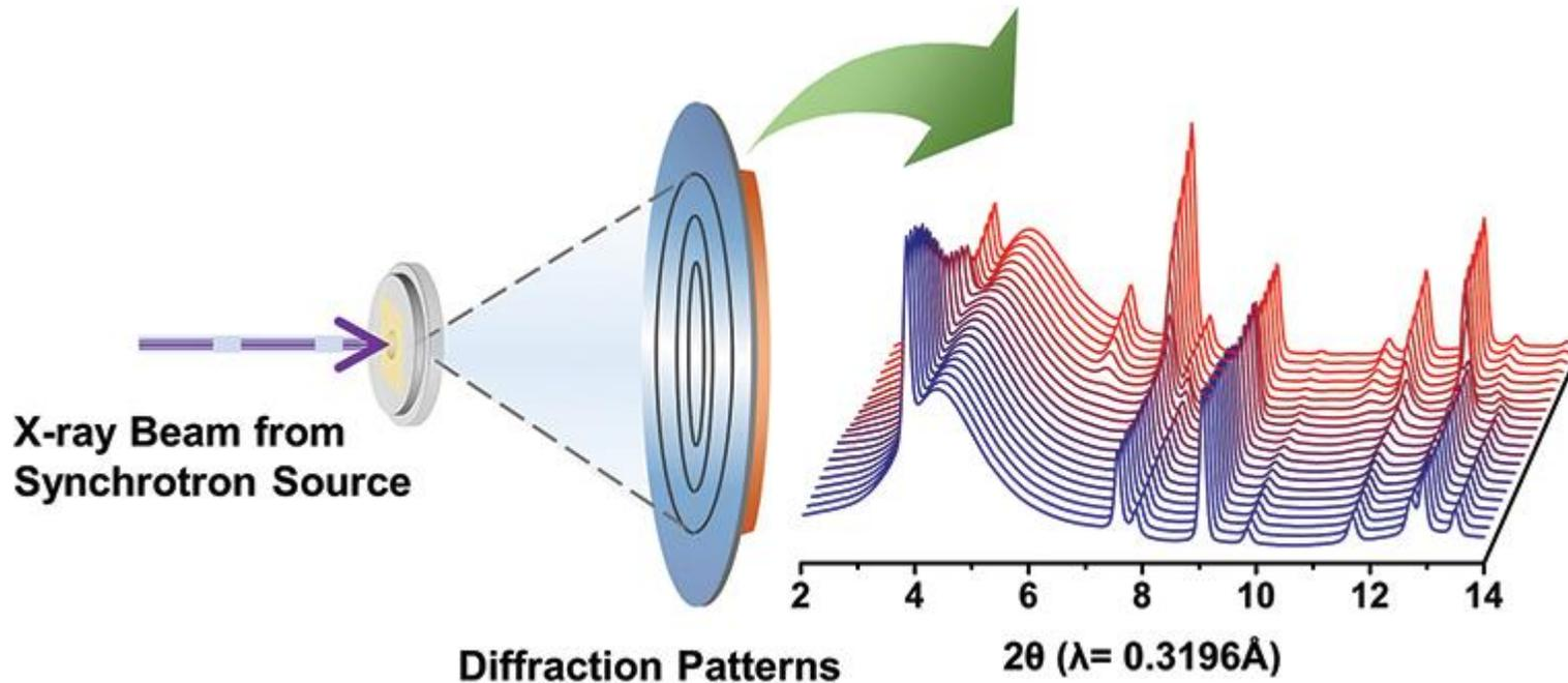
The use of high energy, sometimes referred to as hard X-rays, is advantageous because these X-rays are not absorbed well in a solid material and therefore allow for deep penetration.
