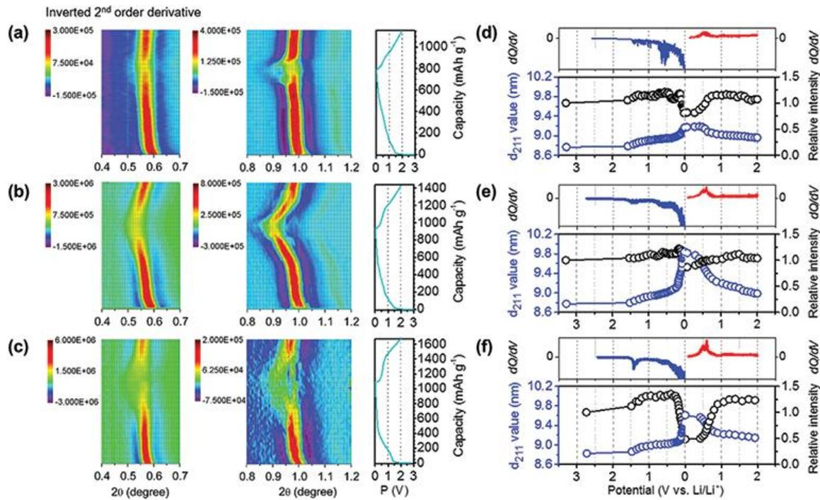
a-c) Color-coded contour projection maps during in situ experiment with corresponding voltage profile and (d-f) the changes in lattice parameters and resolved peak-relative intensities with the corresponding dQ/dV plot for meso-Co<sub>0.5</sub>Sn<sub>0.5</sub>, meso-Co<sub>0.3</sub>Sn<sub>0.7</sub>, and meso-Co<sub>0.1</sub>Sn<sub>0.9</sub>, respectively.
