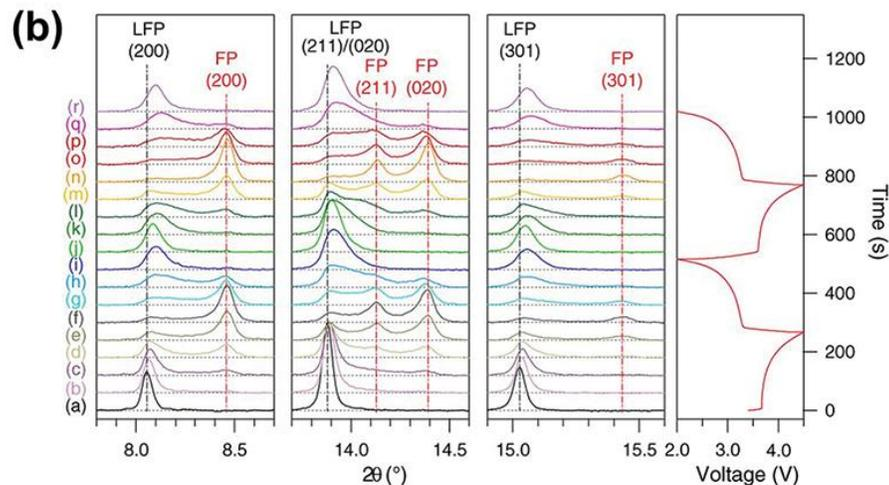
The variations of XRD pattern during the galvanostatic charge and discharge at a rate of 10 C.
