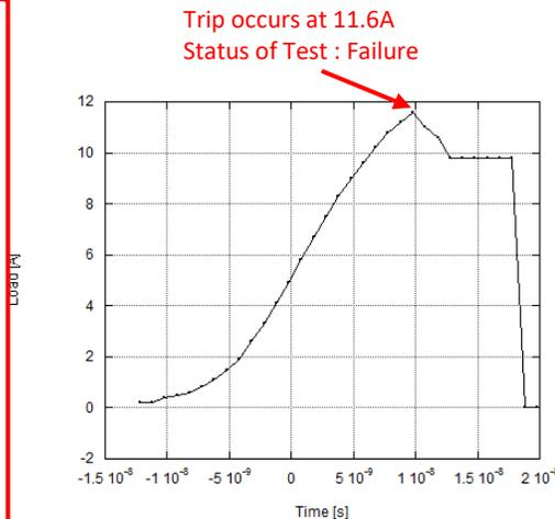
Fig. LVPS Brick over current protection test illustrating a failure.
