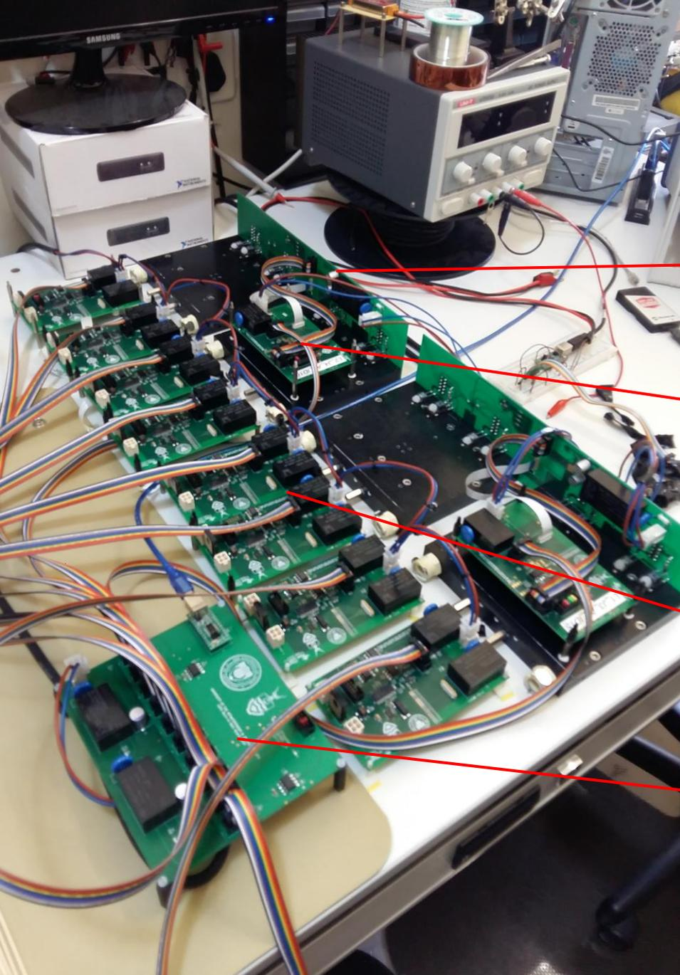
*Fig. Testing of the WITS Burn-in station before final integration with the chassis and cooling system..*
