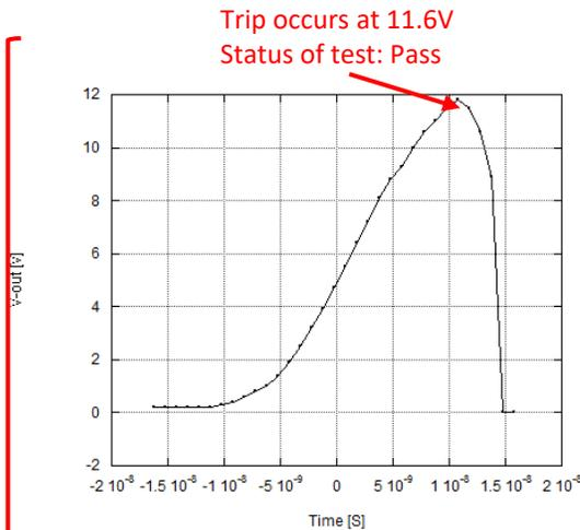
Fig. LVPS Brick over voltage protection test illustrating a pass.
