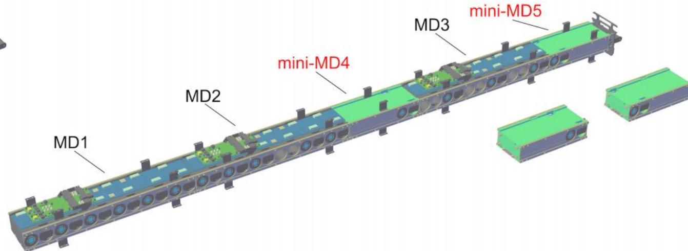
Fig. Super-drawer architecture designed explicitly for Extended Barrels modules, ATL-TDR-028 · LHCC-2017-019, pg 70
