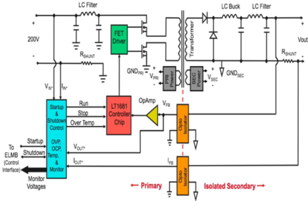
Fig. Block diagram of the LVPS Brick. ATLAS-TDR-028 pg 115
