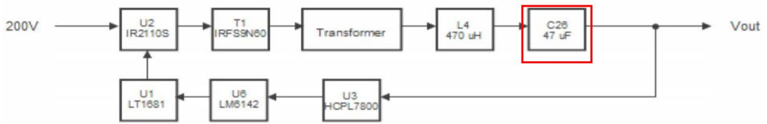
Fig. LVPS Brick simplified signal flow diagram.
