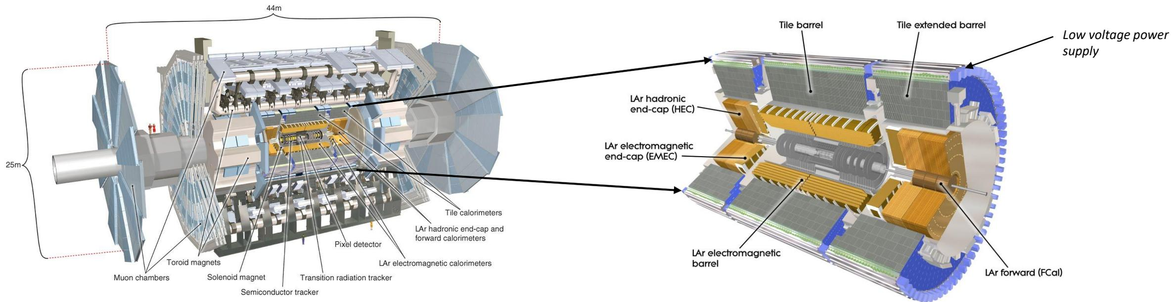
*Fig. Left - The ATLAS detector, Right - The ATLAS inner Barrel, Right*
