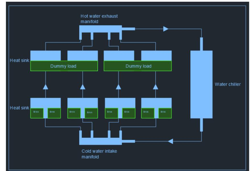
*Fig. Brick Burn-in station cooling system block diagram.*
