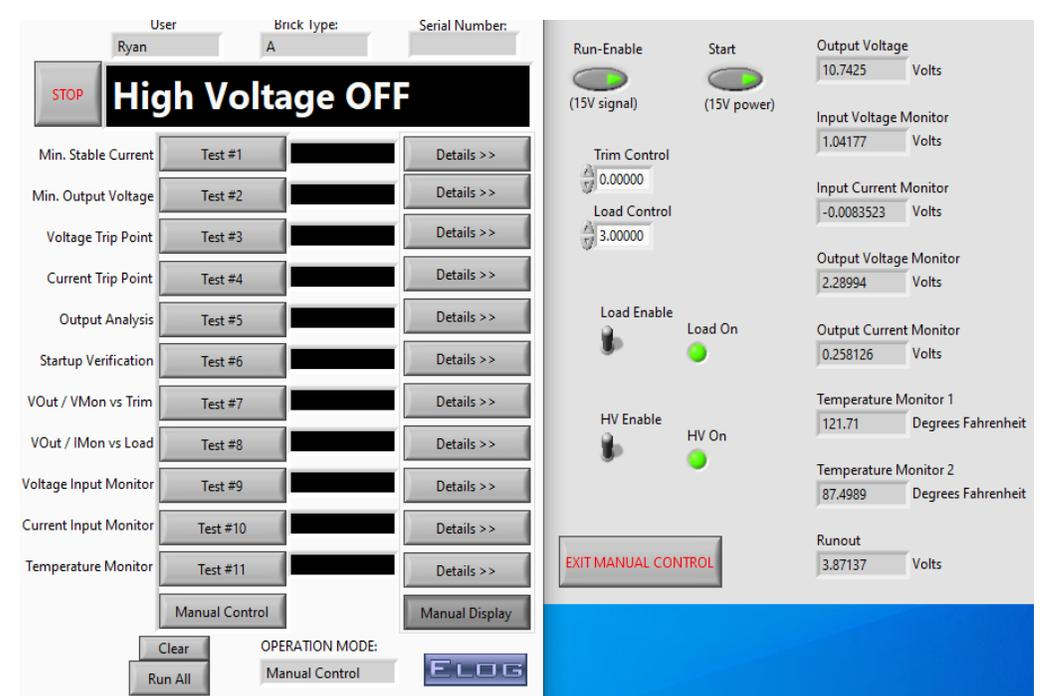
**Fig. Wits Initial test station LabVIEW control program**
