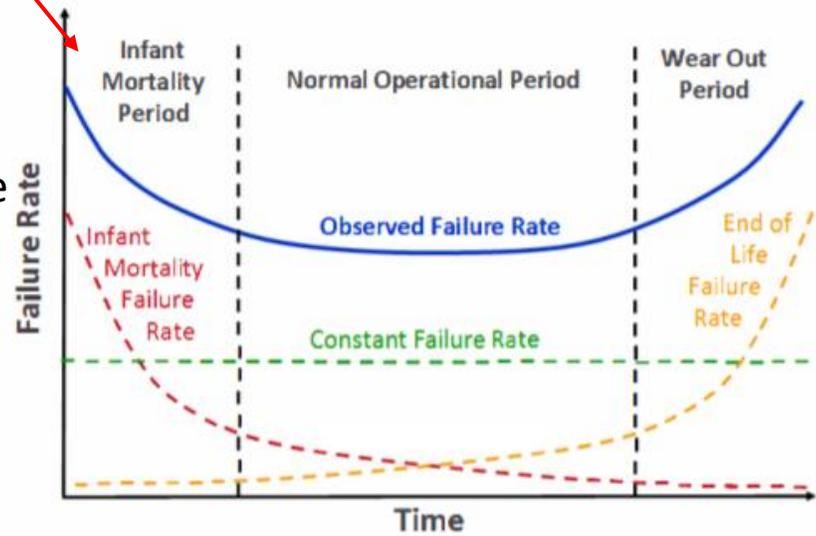
Fig. Bathtub curve of electronics failure rate.
