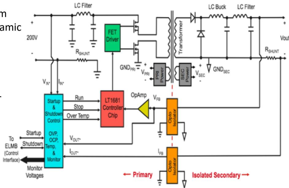
Fig. LVPS Brick functional block diagram.
