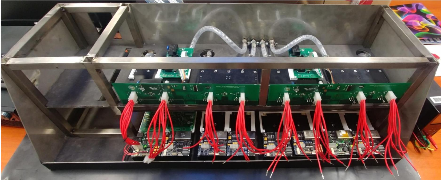
*Fig. LVPS Brick Burn-in station under construction.*
