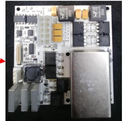
Fig. South African High efficiency LVPS Brick top view.
