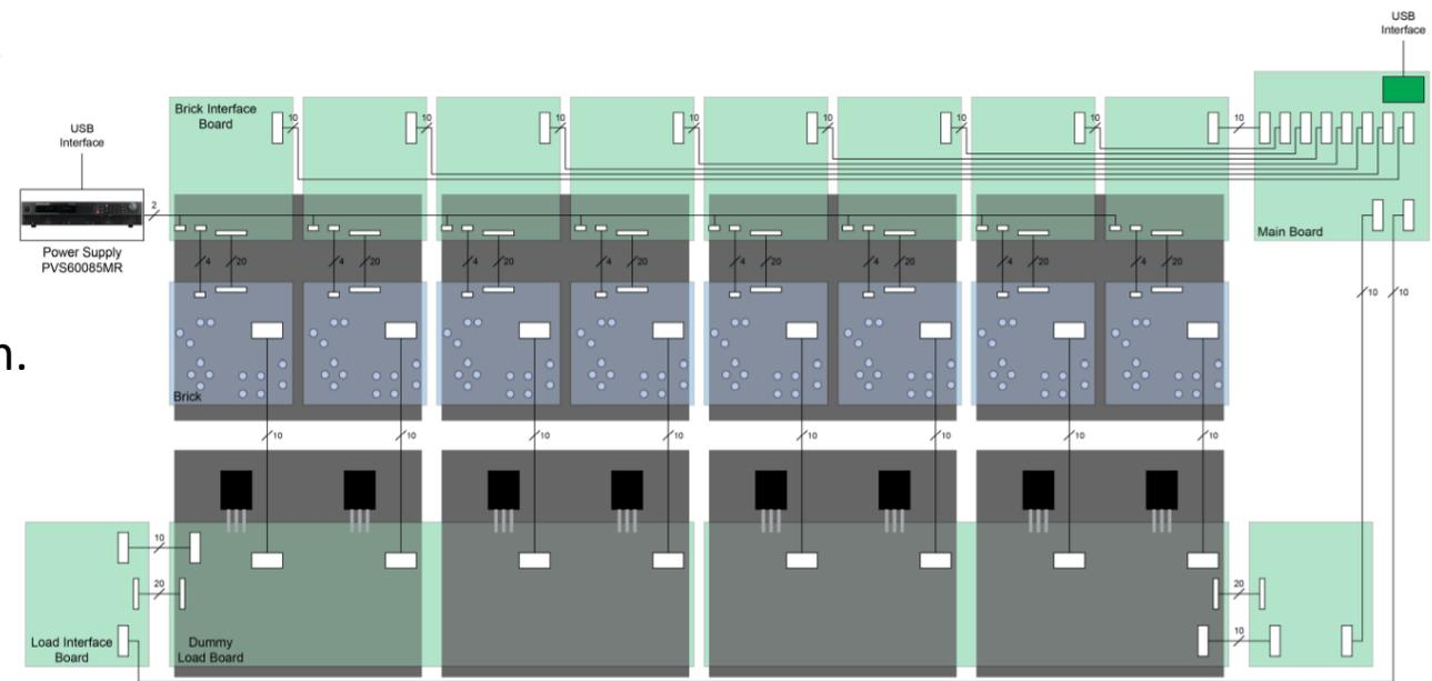
*Fig. Brick Burn-in station block diagram. Seyedali Moeyedi*
