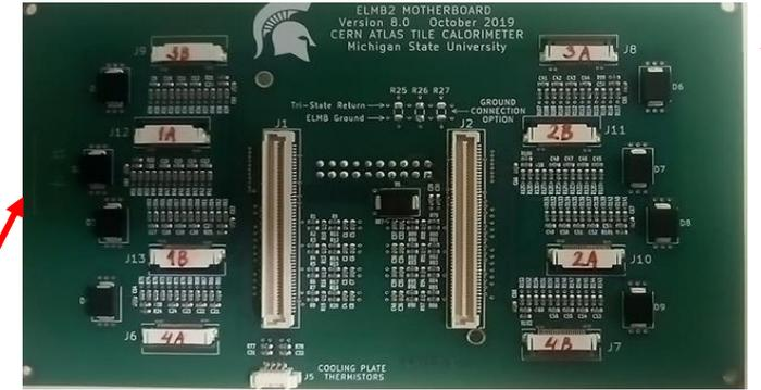
Fig. Embedded Local Monitoring Board
