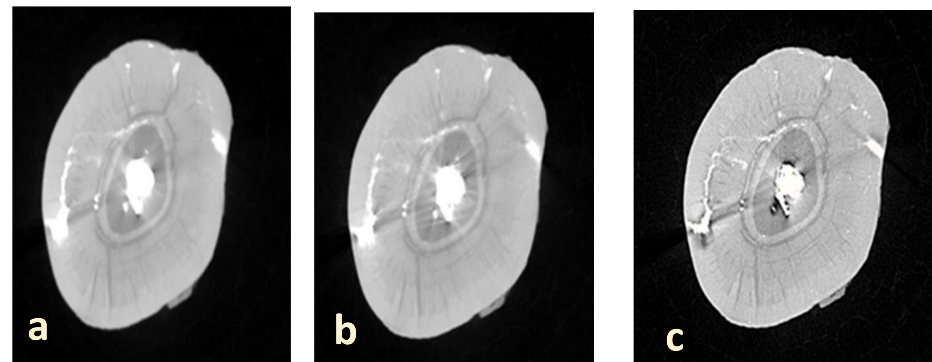
Figure 3: Shows a cross-sectional view of the specimen at slice 985 after applying (a) Gaussian smoothing, (b) median, and (c) unsharp mask filter respectively.
