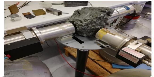
The kimberlite is placed in between the three High Purity Germanium Detectors for time differential detection after irradiation for 10 minutes and also a cool down period.
