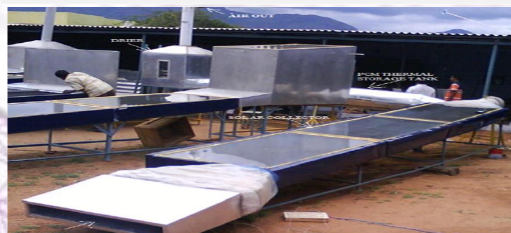
Figure 3: A double pass V-corrugated solar air collector
