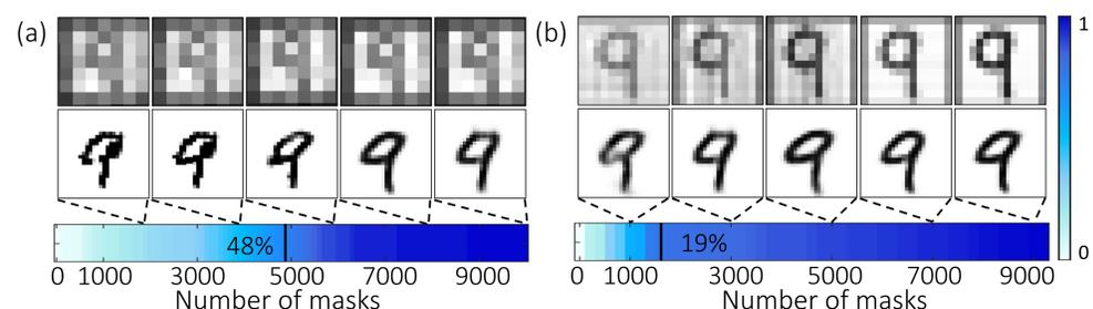
Figure 6: Raw reconstructed images, enhanced autoencoder images and compact confidence curves for (a) 48 x 48 pixel image from 10000 random masks and (b) 96 x 96 pixel image from 9216 Walsh 2D masks.
