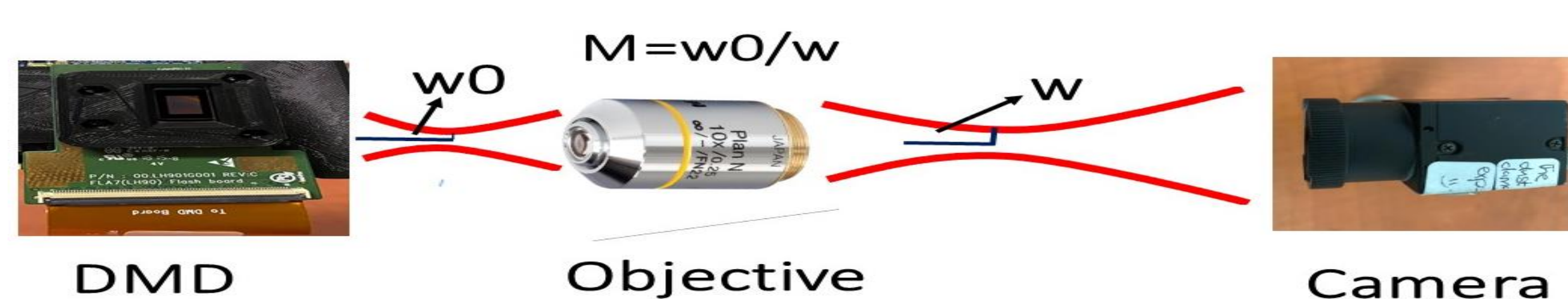
Figure 3: Schematic of the setup used to verify the objective lens placement
