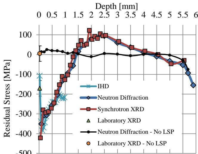
Depth-resolved residuals stress results in the x-direction obtained from multiple methods on the 6 mm and 1.6 mm thick samples
