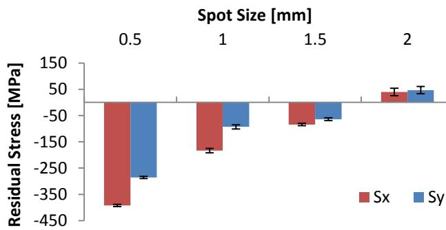
Effect of Power Intensity at IPS = 11.25 for different spot sizes
