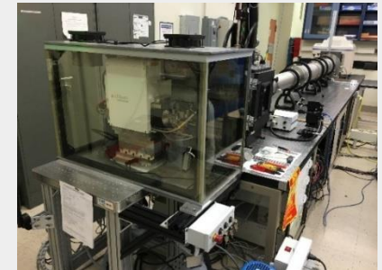
Home-built SAXS system at National Institute of Standards (NIST), USA.
