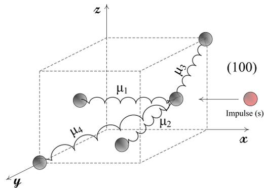
**Figure 2.** Homogeneous mass-spring analogy of FCC structure.
