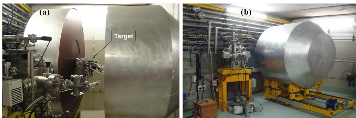
Figure 6. (a) The shielding of the bombardment station in an open position, showing the location of the target on the beamline. (b) The bombardment station in beam-ready state.
