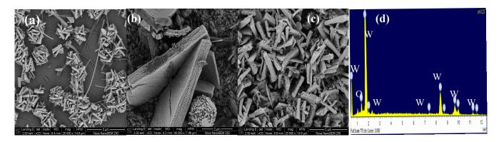
Figure 1.SEM of WO<sub>3</sub> on Corning glass prepared at (a) pH=0.23; (b) pH=0.44; (c) pH=0.91; (d)EDX spectrum of WO<sub>3</sub> on CG.
