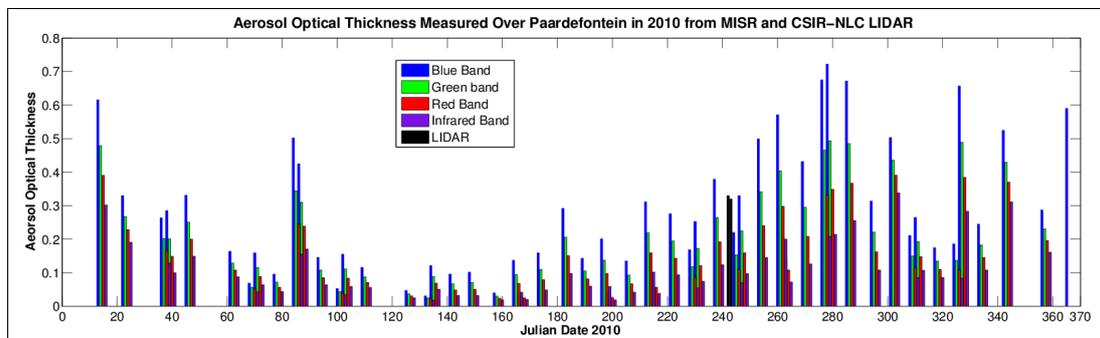
Figure 8: AOT measured by MISR and average AOT obtained from CSIR-NLC mobile LIDAR in the Green band.
