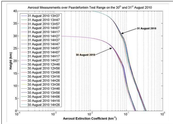
Figure 5: Aerosol extinction coefficient retrieved from LIDAR returned signal for the 30<sup>th</sup> and 31<sup>st</sup> August 2010.
