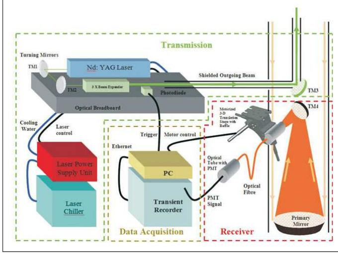
Figure 1: Detailed system block diagram showing all the CSIR-NLC mobile LIDAR components [4].
