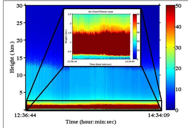
Figure 6: Height-time-colour map of LIDAR signal (glued analog and photon count) returns for the 31<sup>st</sup> August 2010
