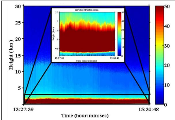
Figure 4: Height-time-colour map of LIDAR signal (glued analog and photon count) returns for the 30<sup>th</sup> August 2010.
