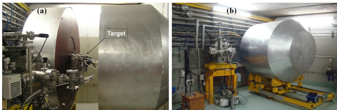
Figure 2. (a) The shielding of the bombardment station in an open position, showing the location of the target on the beamline. (b) The bombardment station in beam-ready state.
