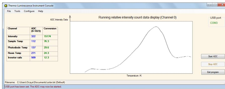
**Figure 6.** TL glow-curve of a polymer sample in the .net program console.
