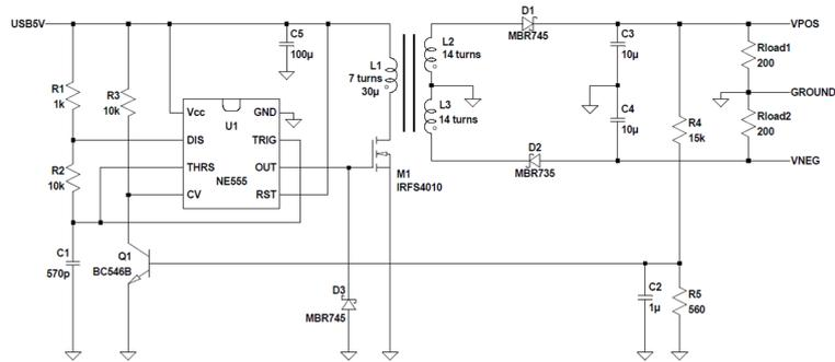
**Figure 5.** Dual-rail amplifier power supply, giving  $\pm 9.26\text{V}$  with the  $200\Omega$  loads shown.
