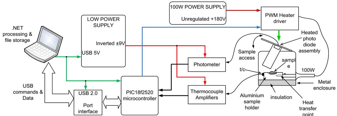
**Figure 1.** Block diagram of the TL system. The thermocouple is labeled “t/c”.
