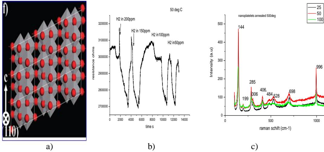
**Figure 1:** a) Arrangement of VO<sub>6</sub> octahedra in real crystalline structure in (010) of VO<sub>2</sub> (A), b) various responses at room temperature for different H<sub>2</sub> concentrations in dry air, c) Raman spectra collected for nanoplatoletsVO<sub>2</sub> annealed at differents output power 25mW, 50mW and 100mW.
