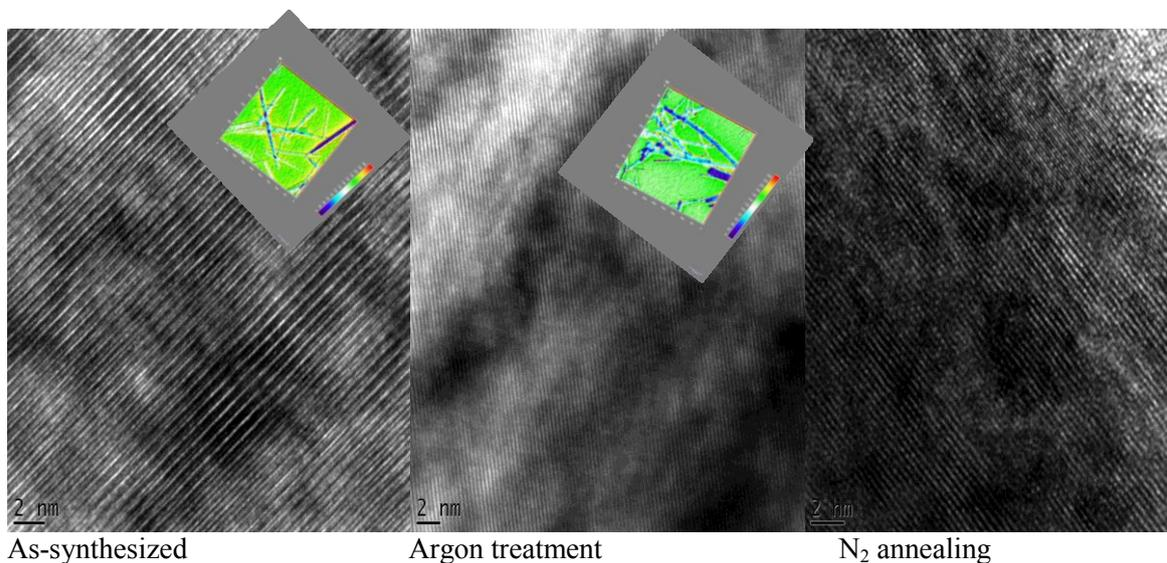
**Figure 4.** Grains structure observed at different annealing gas.
