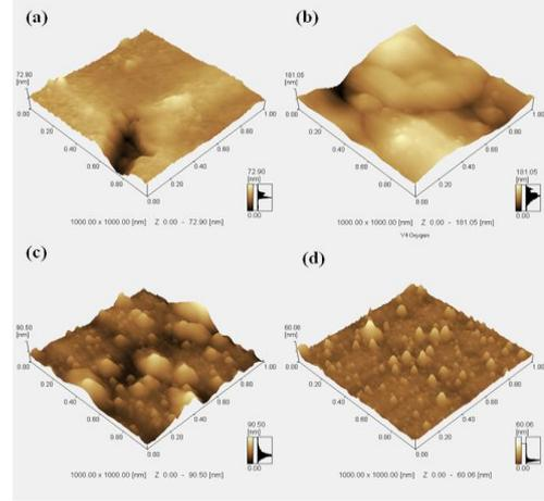
**Figure 2.** Three dimensional AFM images, for the thin film surfaces, grown in (a) base, (b) O<sub>2</sub>, (c) Ar and (d) N<sub>2</sub> atmosphere.
