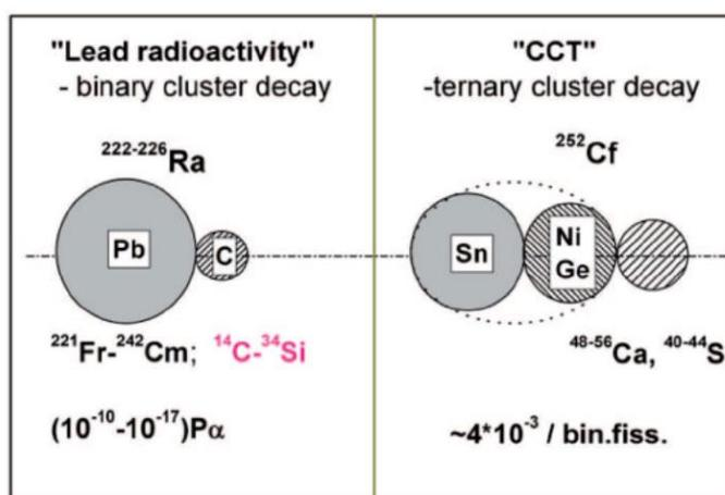
**Figure 6.** Comparison of lead radioactivity on the left with collinear cluster tripartition on the right [2]
