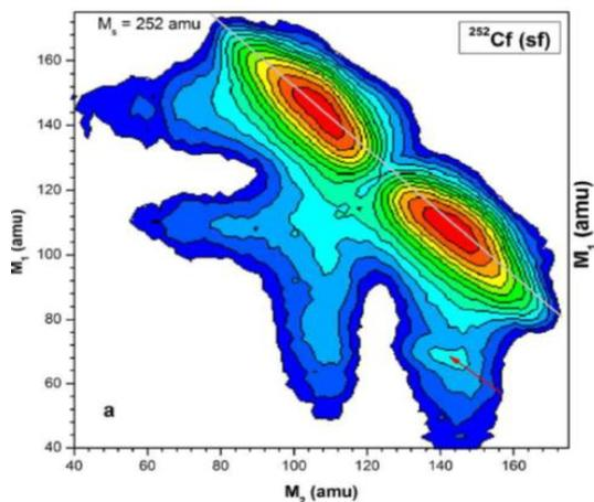
**Figure 4.** Contour map (in logarithmic scale) of the mass-mass distribution of the collinear fission fragments of  $^{252}\text{Cf}$  detected in coincidence in the two opposite arms of the FOBOS spectrometer [2]
