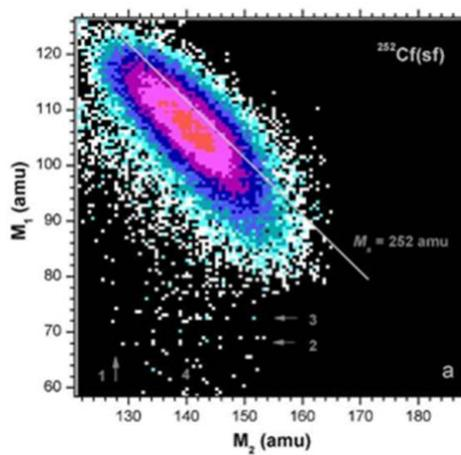
**Figure 5.** The region of the mass-mass distribution for the fission fragments of  $^{252}\text{Cf}$  around the CCT bump with no additional gating [3] and [5].
