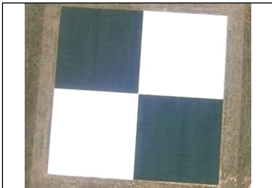
Figure 1. A knife-edge target for measuring the MTF of satellite imaging systems.
