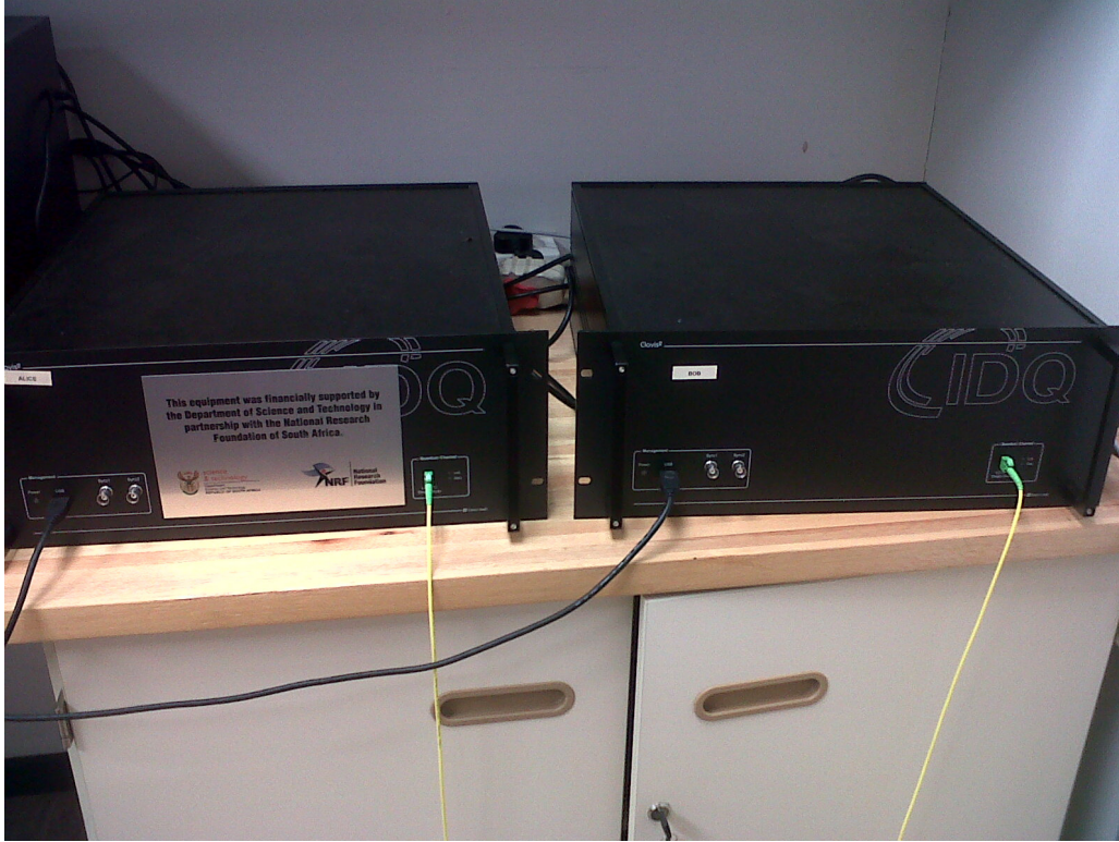
Figure 3. Clavis 2 QKD system in our laboratory at the University of KwaZulu-Natal. Bob's side is on the left while Alice's side is on the right.
