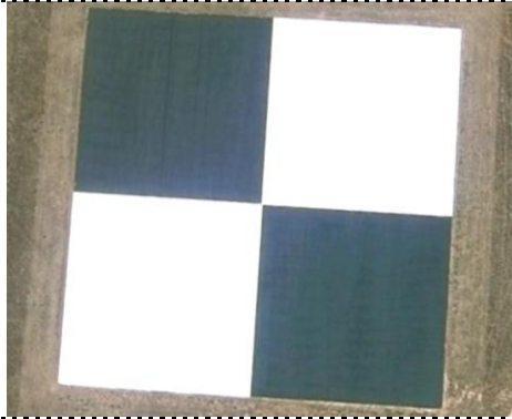
Figure 1. A knife-edge target for measuring the MTF of satellite imaging systems.
