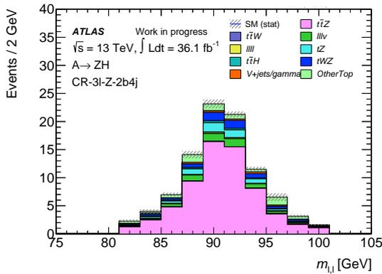
**Figure 3.** Invariant mass of  $Z$ -like lepton pair after the selection of at least four jets with at least two  $b$ -tagged jets.
