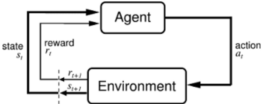
**Figure 1.** A typical setting for reinforcement learning paradigm. An agent interacts with the environment by taking an action based on the state of the environment. In return, the environment rewards the agent. The ultimate goal is the maximization of cumulative reward by the agent.
