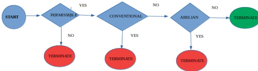
**Figure 2.** A sequence of decision-making steps that the model-free reinforcement learning algorithm takes to search for Majoranas. First, it tests whether the state of matter is physically permissible or not. Then it tests whether the state is conventional or topological. Further, it tests whether exchange statistics are Abelian or non-Abelian.
