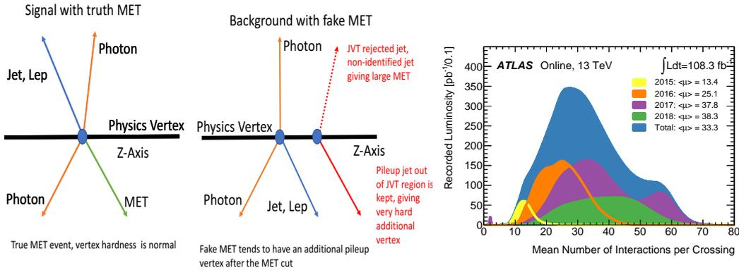
**Figure 1.** Real and fake missing transverse energy in ATLAS experiment.
