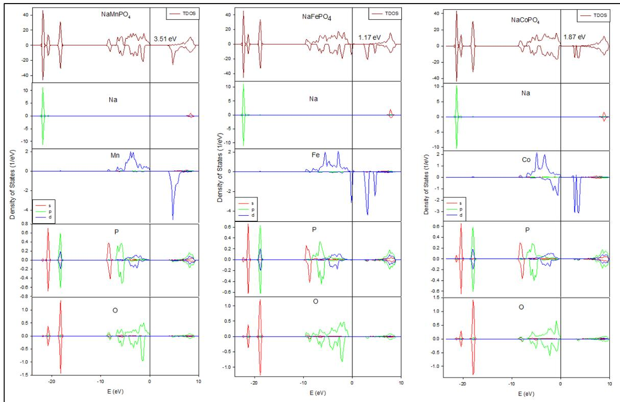
Figure 2 Partial and total density of states plots of olivine NaMPO<sub>4</sub> structures.
