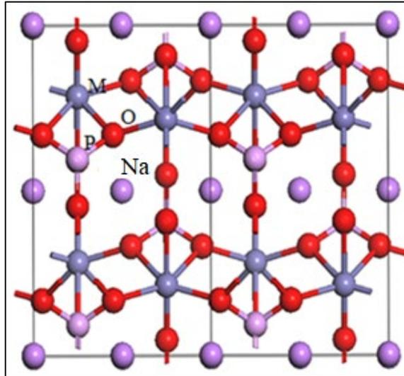
**Figure 1** Atomic arrangement of NaMPO<sub>4</sub> olivine structures.
