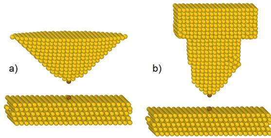
**Figure 1.** (Colour online) The initial configurations used in the simulations: a) a nearly perfectly shaped conical tip above an adatom on a clean surface, and b) a tip that was obtained by repeated rupture and contact formation of a notched nanowire, above the same surface with the adatom. Both tips are oriented along the (001) crystallographic direction, while the surface has a (111) orientation.
