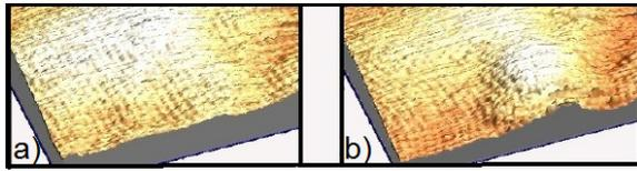
**Figure 3.** (Colour online) The formation of a mound on a gold surface (20nm x 10nm in dimension) before (a) and after (b) repeated contact formation at 4.2K between a STM tip and a clean surface, both made of 99.995 percent gold (of unknown crystallographic orientation) [34].
