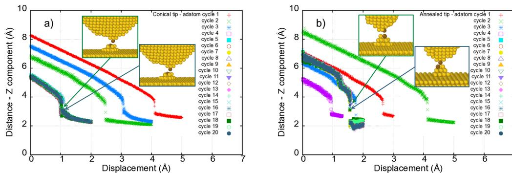
**Figure 2.** (Colour on-line) Minimum distance between the tips and surface versus bulk tip displacement for: (a) a cone-shaped tip oriented along the (001) direction, with its lowest atom positioned directly above an adatom in a three-atom hollow on the (111) surface, and (b), a (001)-oriented tip obtained by (simulated) cyclic loading of a notched nanowire, with its lowest atom positioned directly above the same surface and adatom as in (a).
