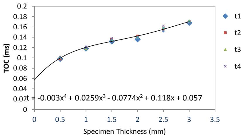
Figure 5. Experimental results: Thickness versus Time of Crossing (TOC).
