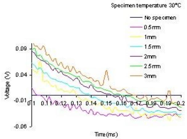
Figure 5. Zero Crossing is Time of crossing (TOC).
