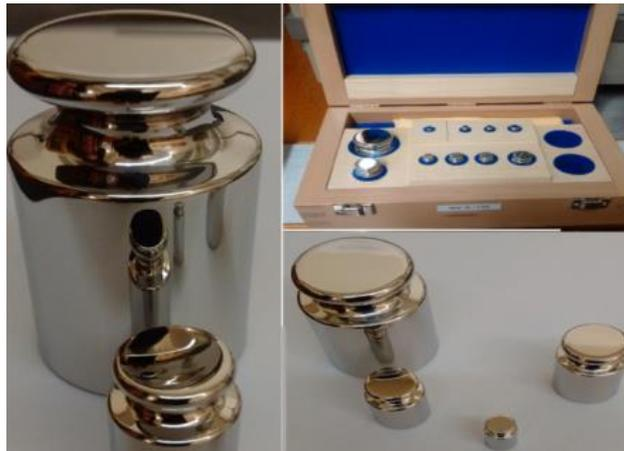
Figure 2: OIML-shaped weights.
