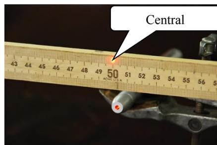
**Figure 2.** Laser experiment – diffraction pattern central maximum.
