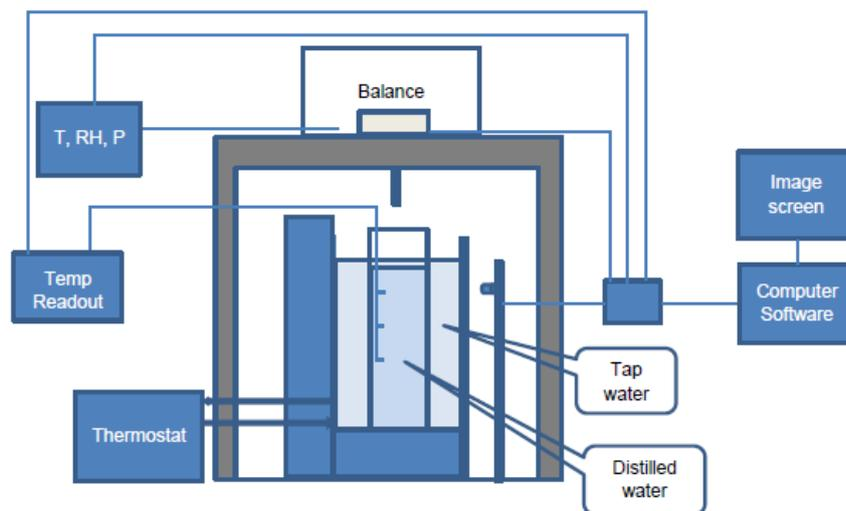
**Figure 2:** A schematic representation of the hydrometer system.
