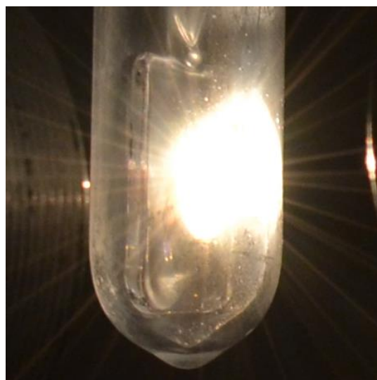
Figure 1. Broadband anti-Stokes white emission observed from graphene upon 975 excitation line in vacuum.
