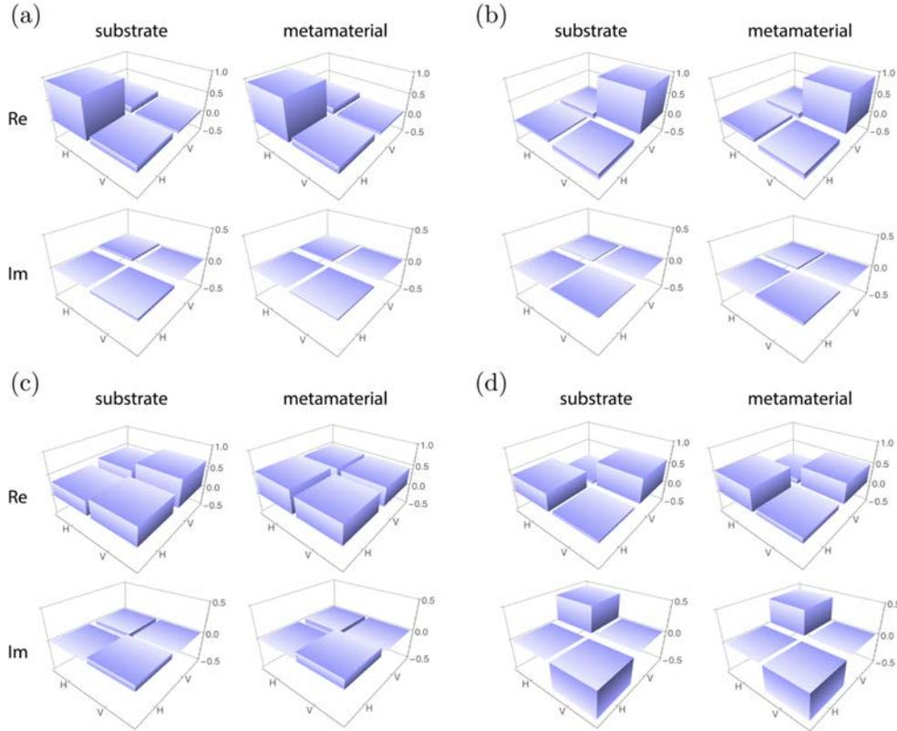
Figure 3: Quantum state tomography of probe states sent through the metamaterial and substrate. (a) Real and imaginary parts of the output state  $\hat{\rho}_{exp}$  obtained from the state  $|H\rangle$  sent through the substrate and metamaterial. (b) Real and imaginary parts of the output state for  $|V\rangle$  sent through the substrate and metamaterial. The other panels show the output states for the following probe states: (c) shows  $|+\rangle$  and (d) shows  $|L\rangle$ .
