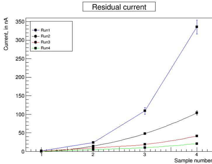
**Figure 2.** Residual current measurements for the composite scintillator.
