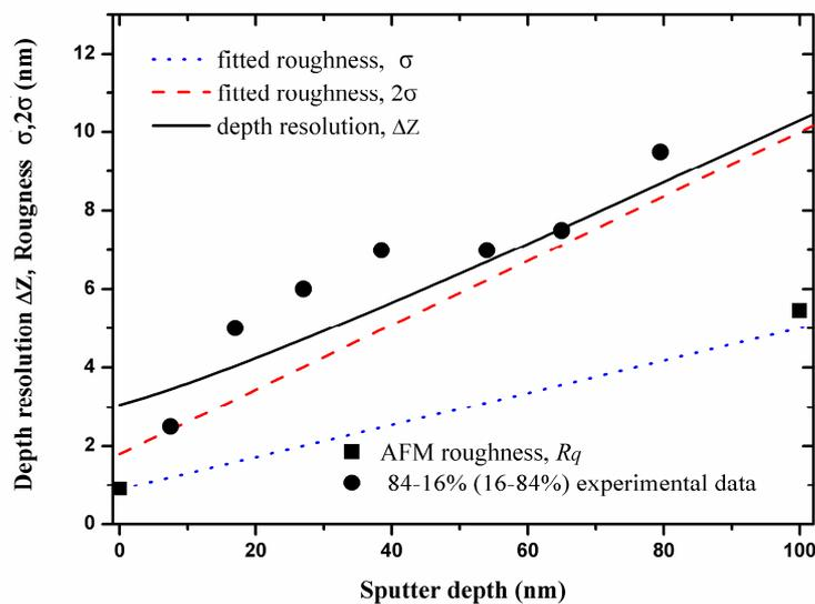
**Figure 4.** The depth resolution  $\Delta z$  (solid line) and the fitted roughness parameter  $\sigma$  and its double value  $2\sigma$  (dotted and dashed lines, respectively) as a function of the sputter depth for the as-deposited sample. The closed circles and squares represent the values of the depth resolution by 84-16% (16-84%) method and the  $R_q$  roughness values determined by AFM (see Fig.1), respectively.
