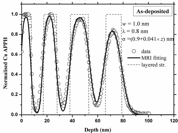
**Figure 3.** The normalised Cu depth profiling data and the best fit to the measured data by the MRI model for the as-deposited sample. The dashed line drawn represents the as-deposited Cu sublayer structure.
