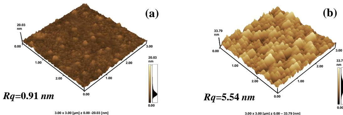
**Figure 1.** AFM images of (a) the surface of the as-deposited sample and (b) the crater centre for sample sputtered at the depth of 100 nm (substrate  $\text{SiO}_2$  surface). The corresponding root mean square (RMS)  $R_q$  roughness values were determined as 0.91 and 5.54 nm, respectively.
