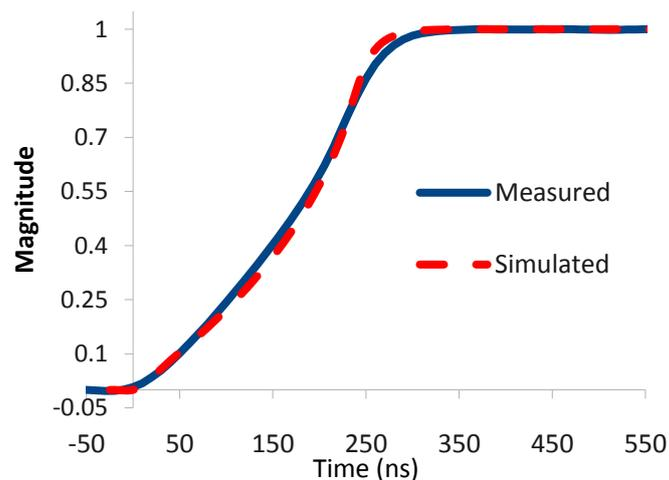
**Figure 5.** Comparison of the experimentally measured (solid) and simulated signal (dash) for the core of crystal A at a position of  $x = 35$ ,  $y = 55$  and  $z = 62$  mm.
