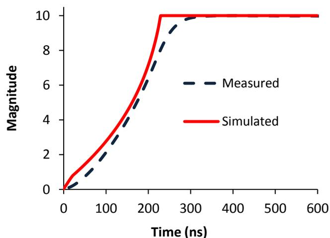
**Figure 1.** ADL simulated signal without the preamplifier response function (solid) and the experimental measured signal (dash).
