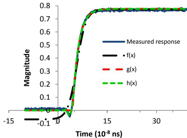
**Figure 3.** The function  $f(x)$  (dash dot) and exponential  $g(x)$  (large dash) function were initially used to fit the measured preamplifier response (solid). The function  $h(x)$  (small dash) includes both exponential and an undershoot.
