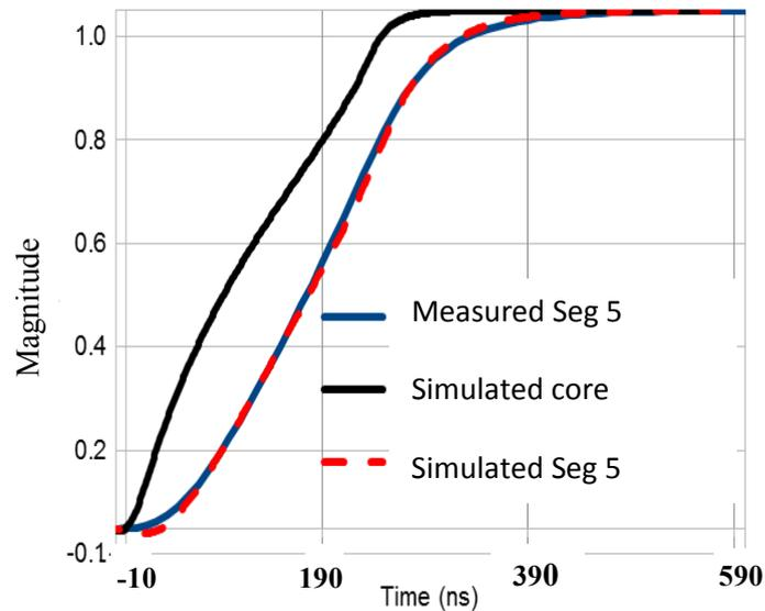
**Figure 6.** Experimentally measured pulse for hit segment 5 (solid blue), ADL simulated pulse with core preamplifier response function (solid black), and simulated pulse with delayed core preamplifier response function (dash red).
