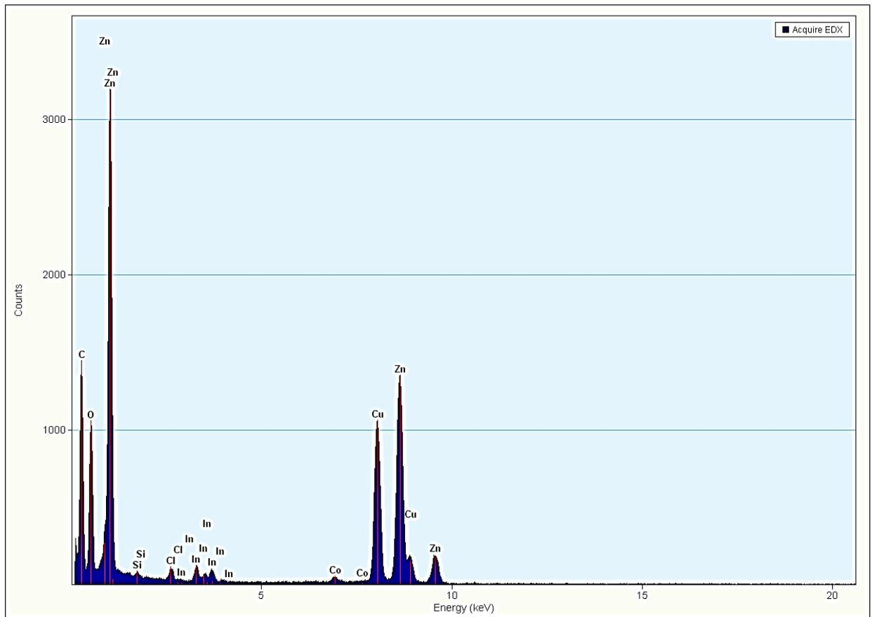
Figure 3. EDS image of 5%In-Co-ZnO nanoparticles.
