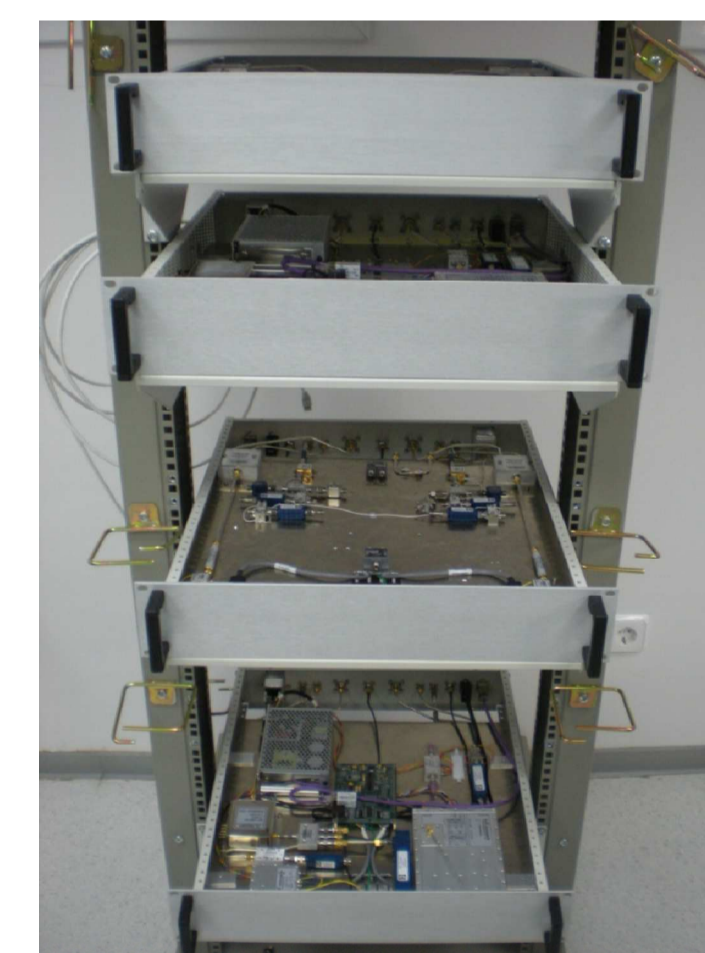
Figure 3b: Up/Down converters integration
