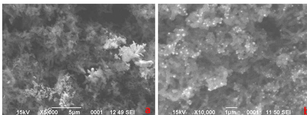
**Fig. 3** SEM images of (a) PANI and (b) Au-PANI composite film
