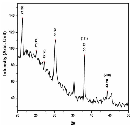
**Fig. 4** XRD pattern of the Au-PANI composite film.
