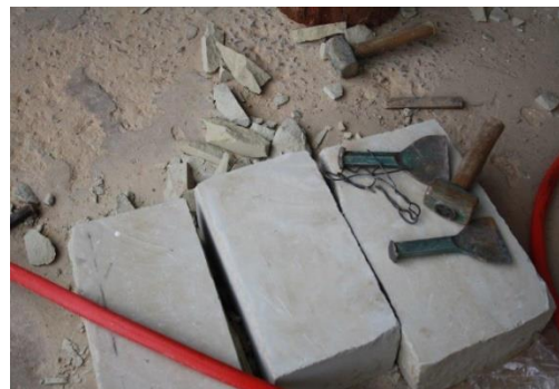
Figure 2. Tools used during the artisanal mining of sandstones.
