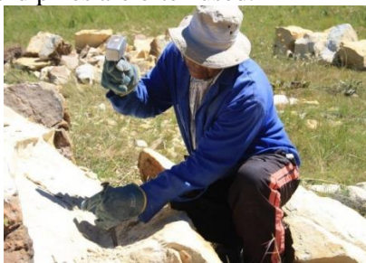
Figure 1. Sand stones are artisanal mining of sandstone is made with hammer, chisels and square
