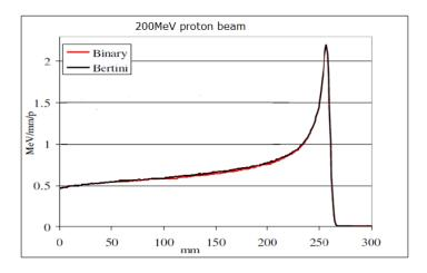
**Figure 2.** Stopping power of a 200MeV proton beam in a water phantom: electromagnetic + inelastic scattering models.
