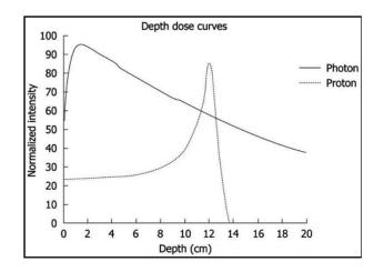
**Figure 1.** Typical depth dose curve for photons and protons as pictured by Studenski & Xiao (2010) [1]
