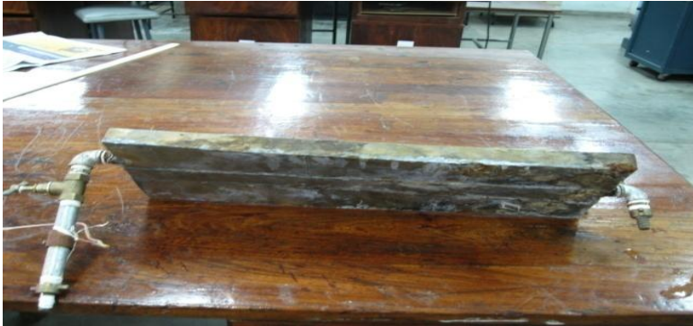
Figure 2.2: The thermal collector tank
