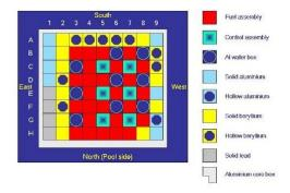
Figure 1: SAFARI-1 reactor core layout
