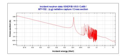
Figure 3: The energy-dependent cross-section of <sup>59</sup>Co
