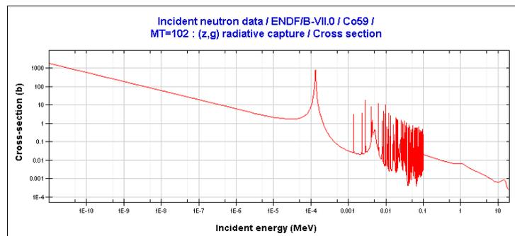
Figure 3: The energy-dependent cross-section of  $^{59}\text{Co}$
