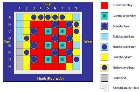
Figure 1: SAFARI-1 reactor core layout
