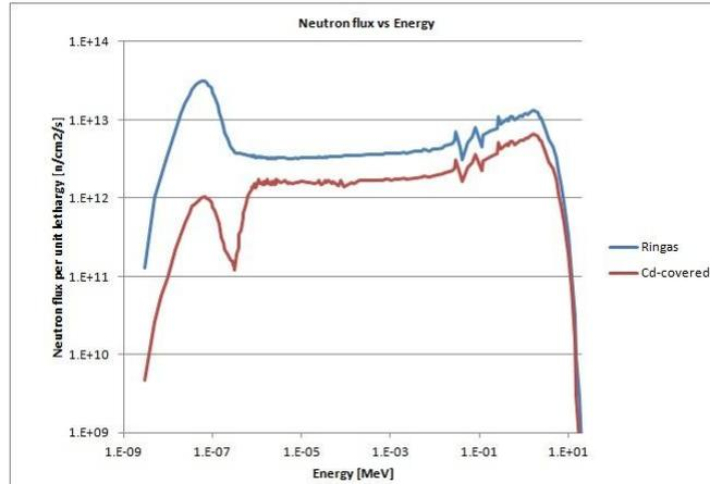
Figure 2: MCNP model of neutron flux
