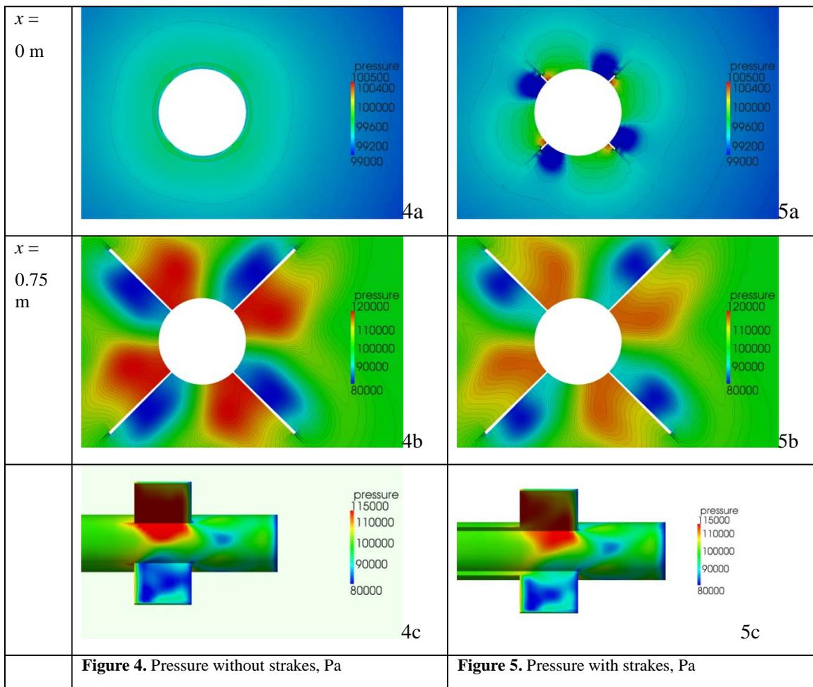
In fig. 4 and fig. 5, pressure contours are compared for the cases with and without strakes. The formation of vortices along the strakes (Fig. 5a) leads to a different structure of the pressure field at the fins (figs. 4b, 5b). Pressure footprints on the fins (figs. 4c, 5c) differ on the forward surface of the leeward fin.
