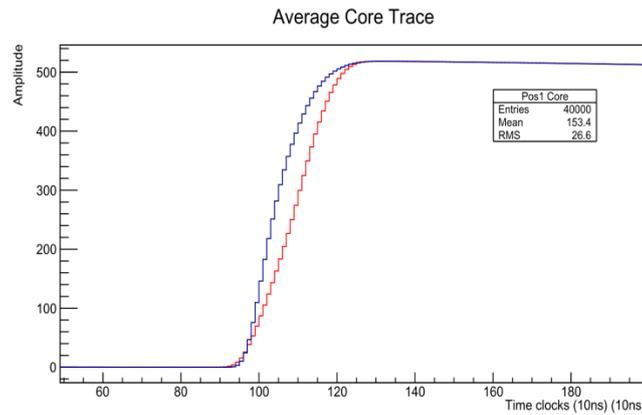
**Figure 4.** The average traces for positions 1 (blue) and 2 (red). The rise times for positions 1 and 2 show a clear difference.
