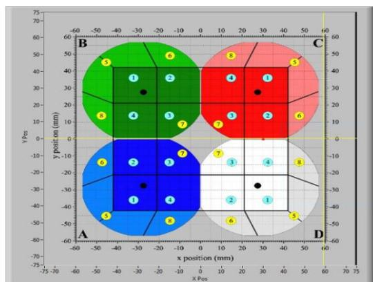
**Figure 1.** Schematic diagram of the HPGe crystals of the iThemba LABS segmented clover detector. The four crystals are labelled as A, B, C, D.
