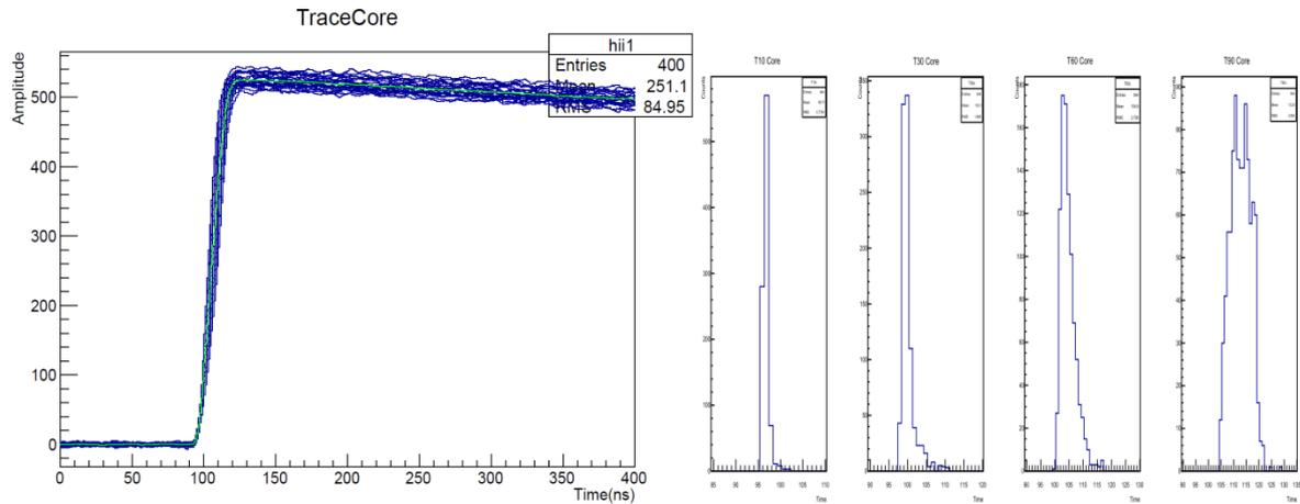
**Figure 3.** Left: The average (green line) and the individual (blue lines) traces for interaction 2, position (-23, 27), which is near the core of crystal B. Right: The measured individual rise times for position 2.
