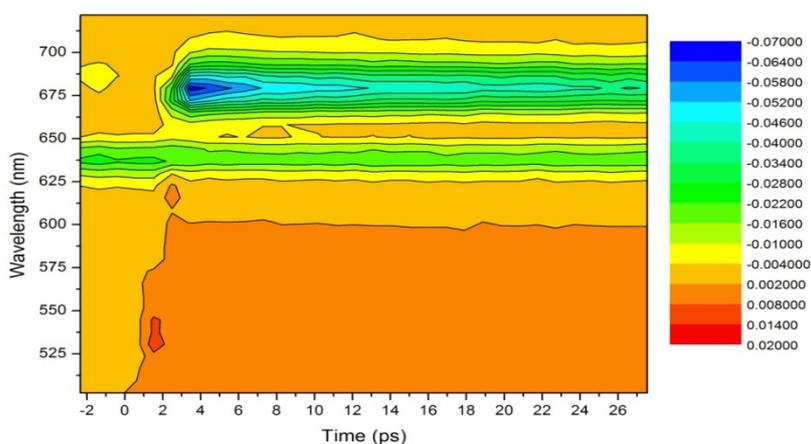
Figure 2: Transient absorption contour plot of ZnPc in DMSO (at a concentration of  $10 \mu\text{M}$ ) pumped at 630 nm, indicating measured absorbance changes for a range of delay times between pump and probe pulses
