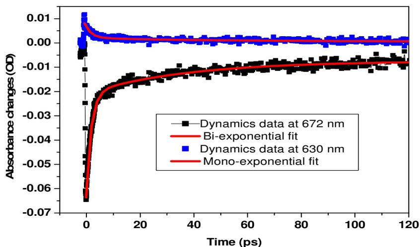
Figure 3: Transient signals of absorbance changes of ZnPc in DMSO at a concentration of  $10 \mu\text{M}$  pumped at 630 nm and probed at 630 nm and 672 nm
