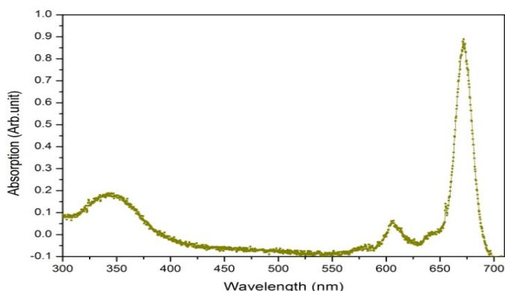
Figure 1: Steady-state absorption spectrum of ZnPc in DMSO at a concentration of  $10 \mu\text{M}$  in a 10 mm path length cuvette recorded using using a Xe-Kr lamp combined with a USB2000 Ocean Optics spectrometer
