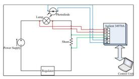
Figure 1. Schematic of Lamp Ageing Experimental Setup
