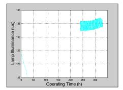
Figure 5. Lamp illuminance drift for 330 hours of operation
