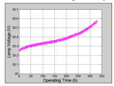
Figure 3. Lamp voltage drift for 330 hours of operation
