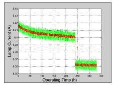
Figure 4. Lamp current drift with associated moving average plot [5] in red for 330 hours of operation
