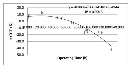
Figure 7. Change in CCT for an Operating Time up to 130 hours
