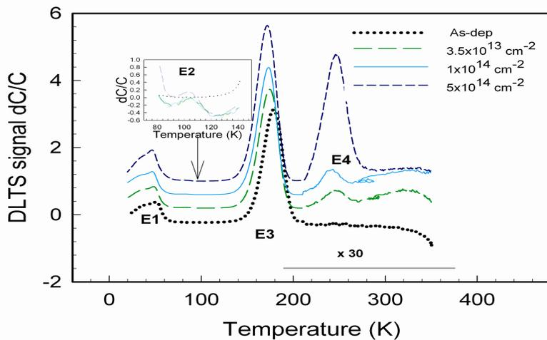
Figure 1: DLTS spectra of as deposited and 1.6 MeV Pd/ZnO Schottky barrier diodes. All spectra were recorded using a quiescent reverse bias 2V, a filling pulse amplitude of 2.2V and filling pulse width of 0.2 ms. The insert shows the E2.
