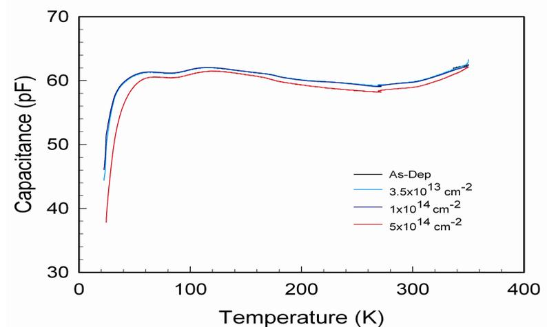
Figure 3: Capacitance-temperature scan obtained as grown and 1.6 MeV alpha-bombarded Pd/ZnO Schottky barrier diodes. The spectra were recorded at quiescent reverse bias of 0V in the 20-350 K temperature range.
