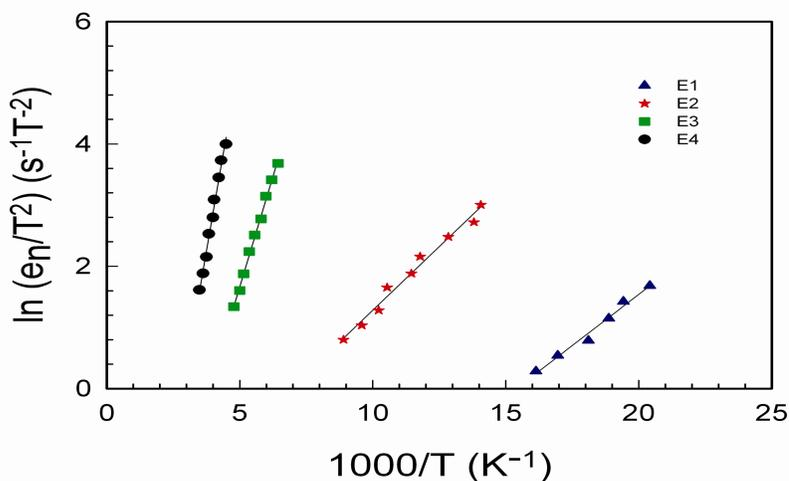
Figure 2: Arrhenius plot obtained from the 1.6 MeV alpha-particle irradiated Schottky barrier diodes.
