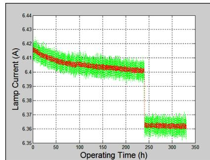
Figure 4. Lamp current drift with associated moving average plot [5] in red for 330 hours of operation
