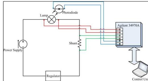
Figure 2. Circuit Diagram of Lamp Ageing Experimental Setup
