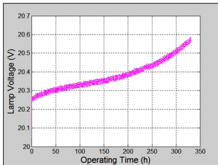
Figure 3. Lamp voltage drift for 330 hours of operation
