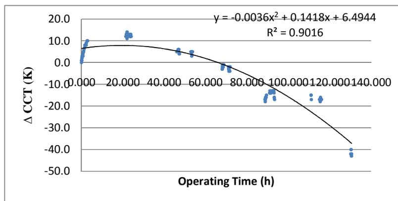
Figure 7. Change in CCT for an Operating Time up to 130 hours
