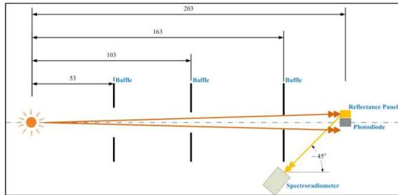
Figure 1. Schematic of Lamp Ageing Experimental Setup
