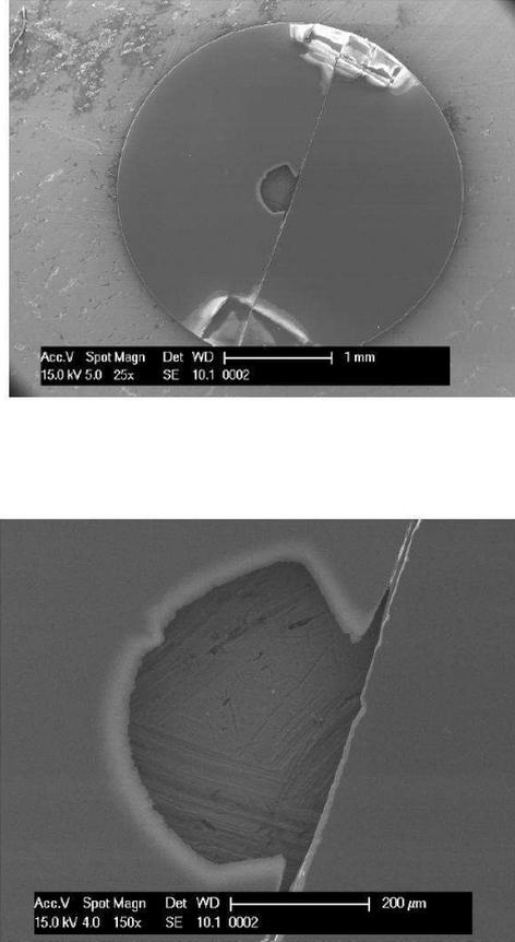
Figure 1: Scanning electron microscope (SEM) images of the cross-sectional ion milled diamond TEM sample. TEM investigation were carried out at the edge of the hole at the diamond/diamond interface.
