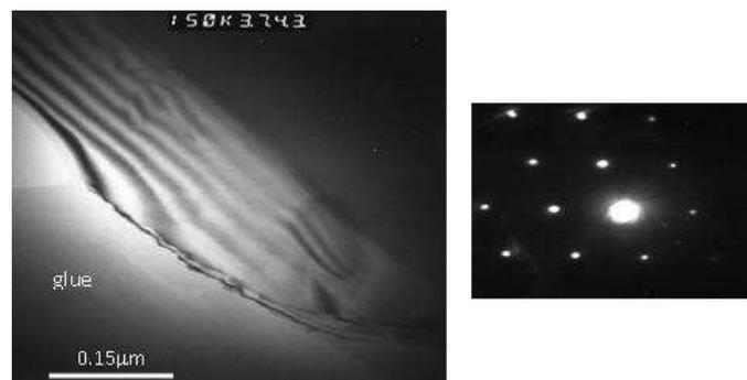
Figure 4: Cross-sectional bright-field TEM micrographs of diamond implanted with carbon ions to a fluence of  $1 \times 10^{15}$  ions  $\text{cm}^2$  with corresponding selected area diffraction pattern. The sample has a thin region (result of ion milling) close to the edge showing a number of thickness fringes.
