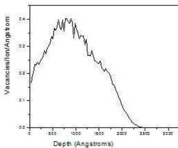
Figure 3: A SRIM-2003 simulation of the damage (vacancy) distribution produced by the carbon ion multi-implantation. The average projected range predicted by the Monte Carlo program is  $\sim 2500 \text{ \AA}$  while the highest level of damage lies at a depth of  $\sim 1000 \text{ \AA}$ .
