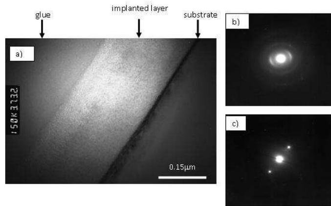
Figure 2: (a) Cross-sectional transmission bright-field TEM micrographs of diamond implanted with carbon ions to a fluence of  $7 \times 10^{15}$  ion  $\text{cm}^2$  at liquid nitrogen and rapidly annealed with SAD patterns from the implanted area (b) and diamond substrate (c). The SAD pattern (b) from the amorphous implanted layer exhibits the 002 arcs of graphite. The SAD pattern in (c) shows the 111 reflections of diamond.
